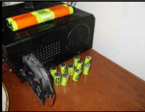
This will be a 10xCP1300 pack so I need 10 individual Nicad batteries arrange as two sticks of 5 cells each.
