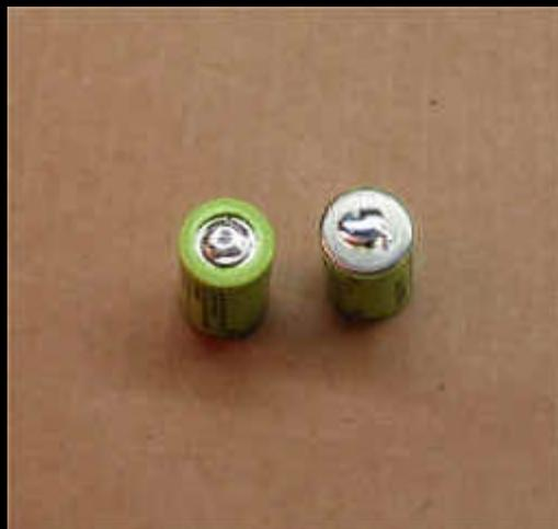
Take some 200 grit sandpaper and lightly sand both ends of each cell. You want to see some scratch marks on it, then wipe the end clean. You want to remove any finish or dirt from it.
