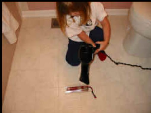
Fire up the hair dryer or heat gun on high heat and shrink away! Remember the heat rule. You are not trying to melt the thing, just shrink it.
