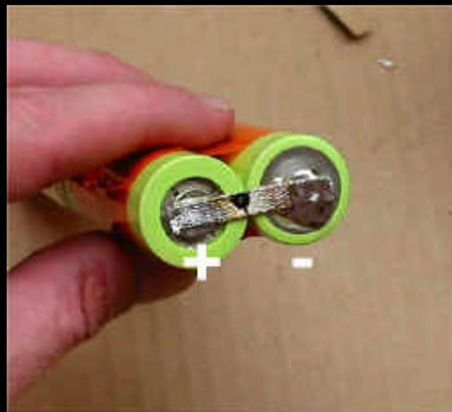
Because of heat concerns, you should tin the end of the braid before attaching it to the cells. This will help minimize the time the soldering iron is in contact with the cells.
