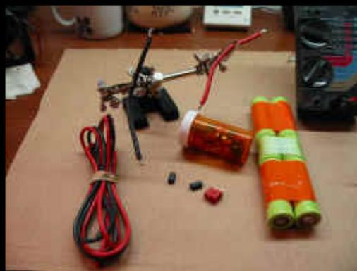
For 10 cells connected in series, another voltage check should reveal roughly 11Volts after the two sticks are connected. Some orange tape helps for visibility.
