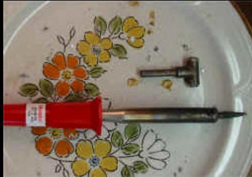
This is a cheap 60W [Hobbico](#) soldering iron that you can find at [TowerHobbies](#). You can purchase a hammer-head tip which helps with soldering packs, or simply find a bolt which fits into the end of your soldering iron.
