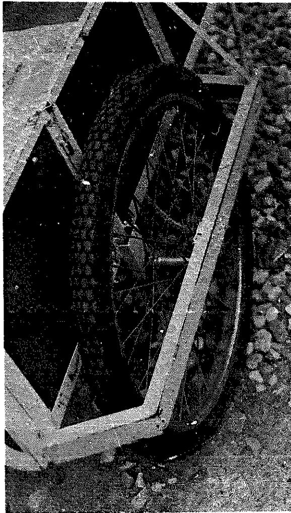
In my experience, bicycle wheels used on carts, not designed for the many shear forces put across the wheels, must be serviced fairly often. The spokes must be kept tight. The bearings and bearing race must be cleaned and repacked regularly, especially since replacement is so expensive.
