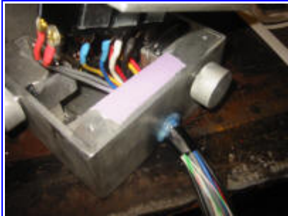
(4) Blue RTV gasket sealer used to seal around the wires before 2 part RTV was poured into place.
