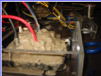
(6) First coat of epoxy and talc is allowed to dry in order to prevent damage from shrinkage.
