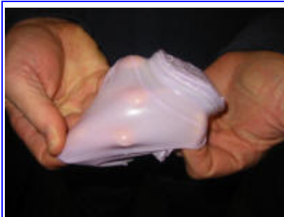
(1) RTV Silicon. Mixed from 2 solutions, it dries in hours and remains flexible.
