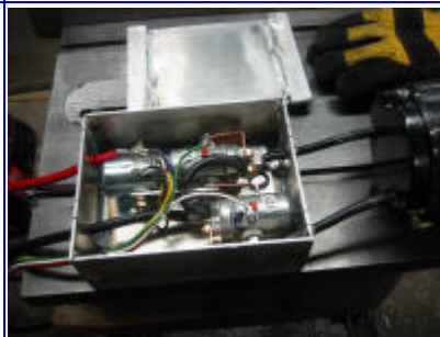
(4) Winch power relay box.
