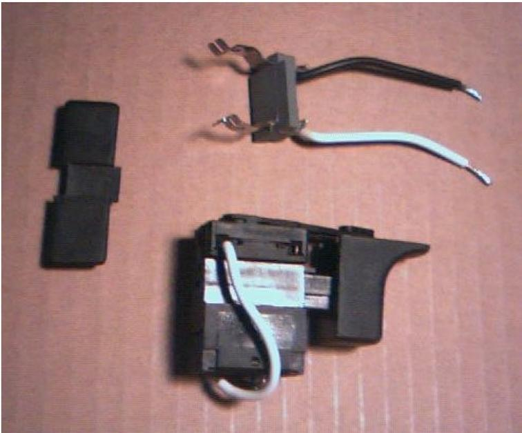
The white wire from the PM motor is positive when cranked counter clockwise facing the chuck and negative when cranked clockwise for the 14.4 Volt drill. There is also an internal 3 wire component (transistor or SRC I don’t know which) that has a heat sink that can sometimes be rewired to act as a diode. Do this in a pinch or emergency, not recommend using if you have a diode available. A diode will work more reliably. For the
