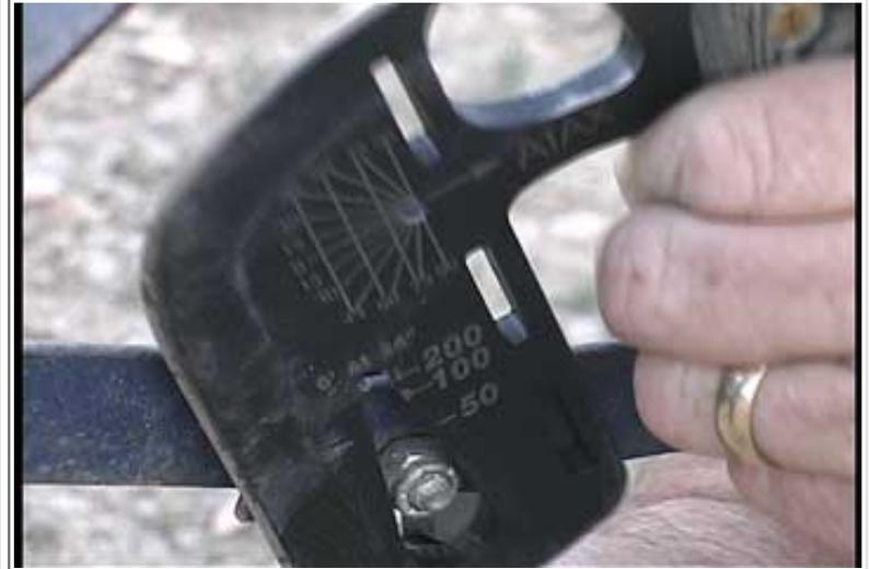
A close up of the ATAX Nut gripper :->
