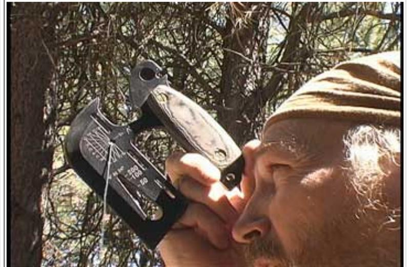
Just sight along the top of the blade and read the angle from the graphic. In the video we show you how to estimate the height of a tree or other object with the ATAX.
