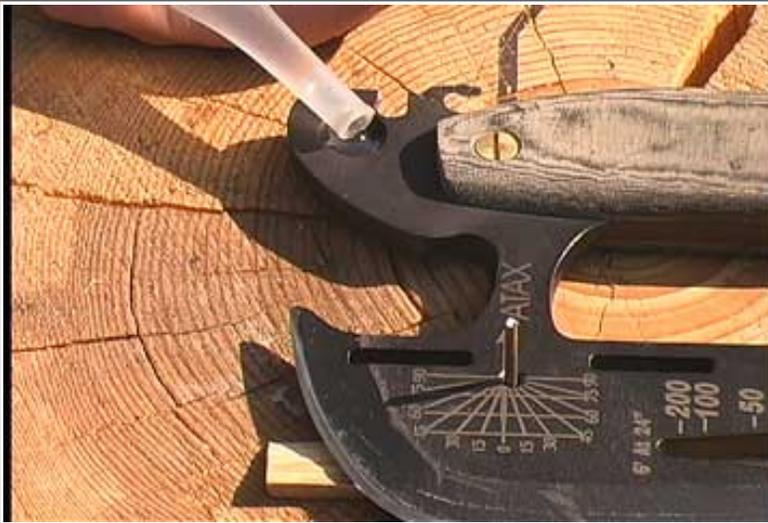
Here you can see the graphic and divot working as a compass/clock. With a twig and a few drops of water you can tell directions and time of day. North is at the bottom of the photo and it is about 4 pm Standard time... That's just the beginning of what you can do with the graphic!
