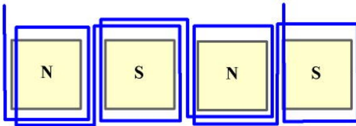
In a single phase unit the coils are wound opposite of the first. That is to say one is wound clockwise and the next is counter clockwise. If your unit has 8 magnets then it would also have 8 coils. With 3 phase you would have 3 coils for each pair
