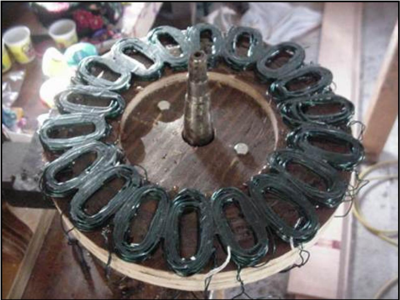
Above is pictured the stator, mostly complete, with the coils smashed down tightly and glued well. At this point, I coated the assembly (plywood front and back) with epoxy to weather proof it as best I could. I divided the coils in half, hooking 2 sets of 9 coils together in series and figured I would decide later whether to hook the two halves in series or parallel - this was not decided until a prop was made and I actually got to test it in known windspeeds.
