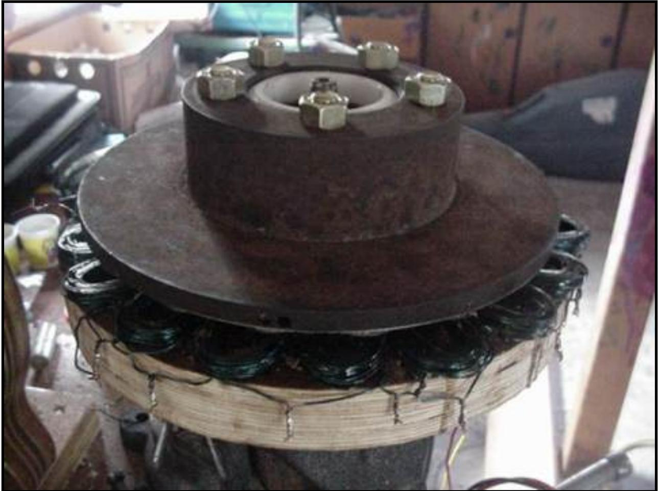
The completed unit. It's already been attached to a homebrew wind generator with an 8-foot diameter, 3-bladed rotor--and is up and flying! [See it HERE!](#) We've already seen peaks of over 60 amps into a 12 volt battery bank, and it survived 60-mph winds last week. Steady output of 30 amps in 28 mph winds, and reaches charging voltage at around 12 mph.
