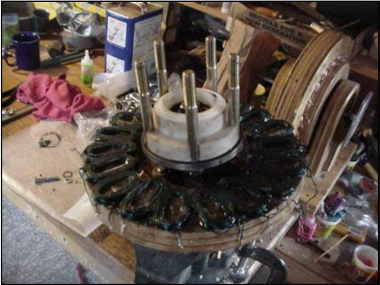
Pictured above, all the parts are assembled except for the armature. Note the long bolts sticking through the hub and spacer. These will hold the rotor on, and the armature will not be held down tightly until the rotor is tightened. Although other systems might work, in this case I decided to lightly tack weld the bolt heads to the wheel hub on the bottom, since it would be impossible to hold them with a wrench once the brake disk (armature) was installed.
