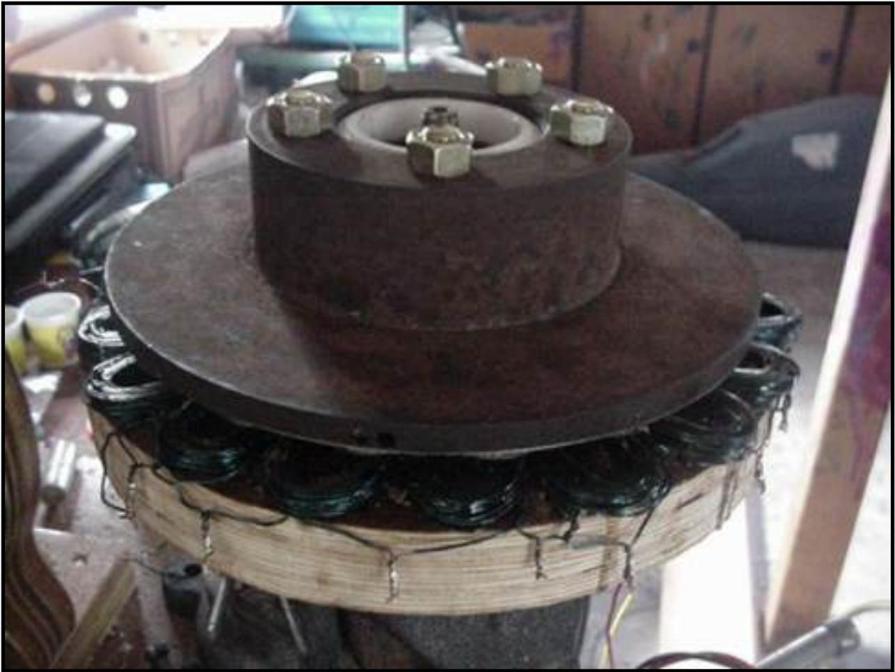
So that's it, all finished up! At this point it becomes obvious that it will be an effective low rpm alternator. There is slight drag from the hysteresis problem of magnetizing the steel bandsaw blade as described above, but it isn't too bad. It spins fairly freely, and when the leads of the stator are shorted out it locks up and becomes very difficult to turn. When the stator is hooked up with all 18 coils in series, it is easy to spin it up to about 15 volts by hand.
