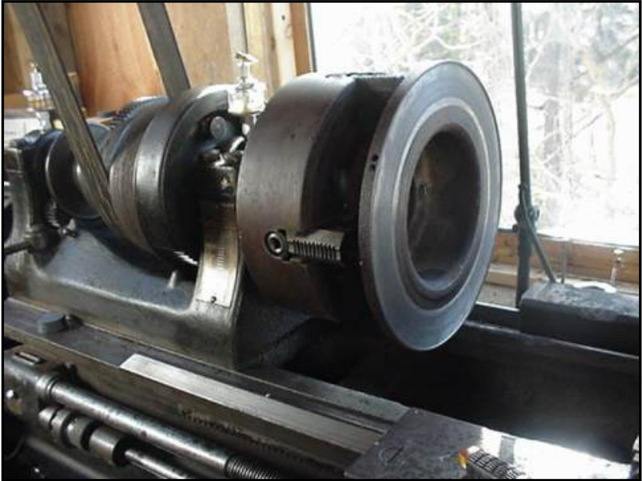
This is the only machine work involved, very easily done by any automotive machine shop, or anybody with a metal lathe. I cut a slot 1.5" wide in the back of the brake disk very near the outer edge. (I left about 1/16" steel on the outer edge) This slot serves to hold the magnets in. It might not be needed, but at high rpm there is risk of the magnets flying off. This slot should hold them in tightly.
