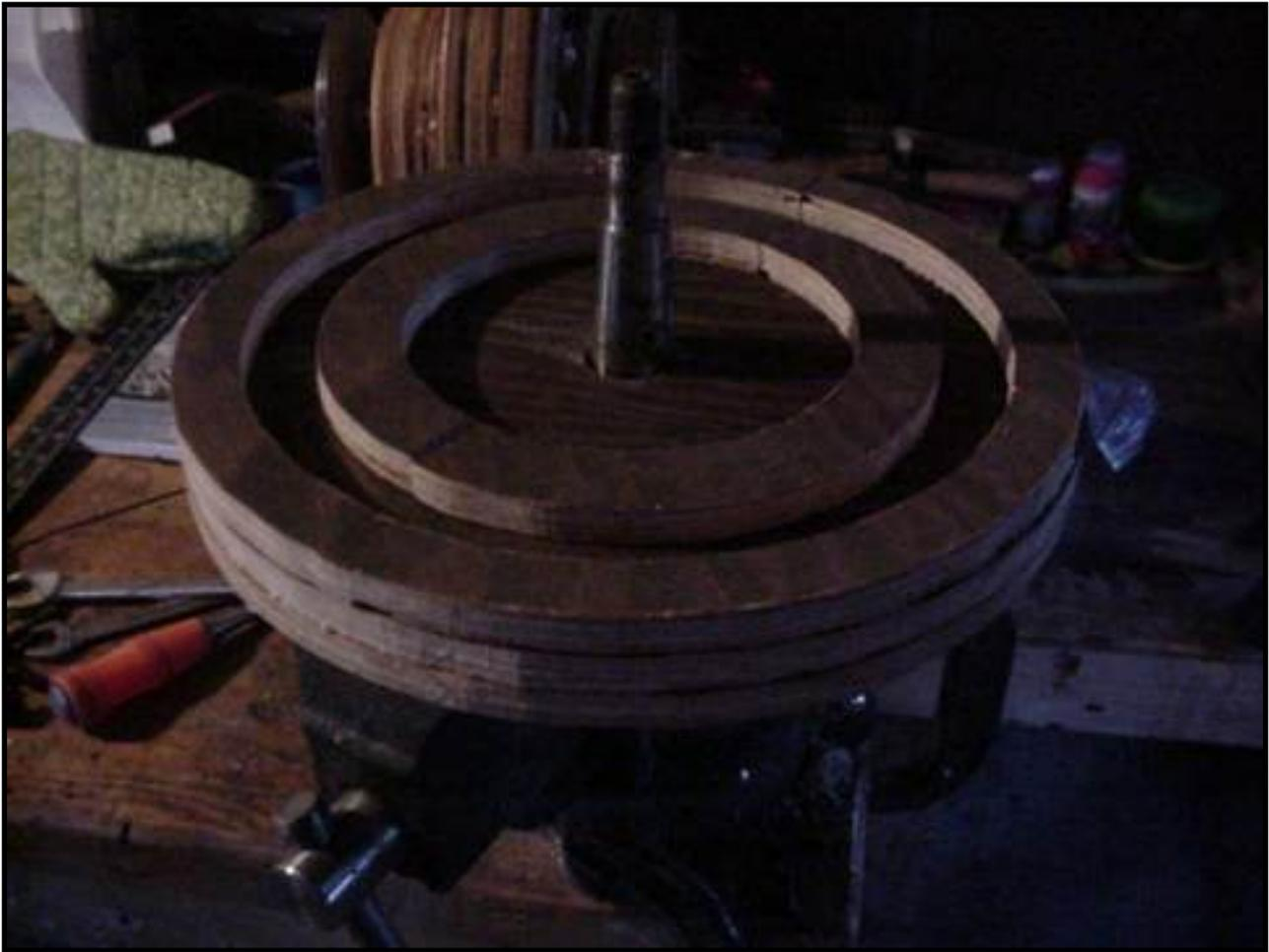
Pictured above is the beginning of the plywood stator. It is made out of laminated plywood discs. The total thickness is 1.5". The top layer, which is 1/2" thick, has a slot 1" wide at about 10" diameter so that steel laminates can be epoxied in. Over that will be the coils.
